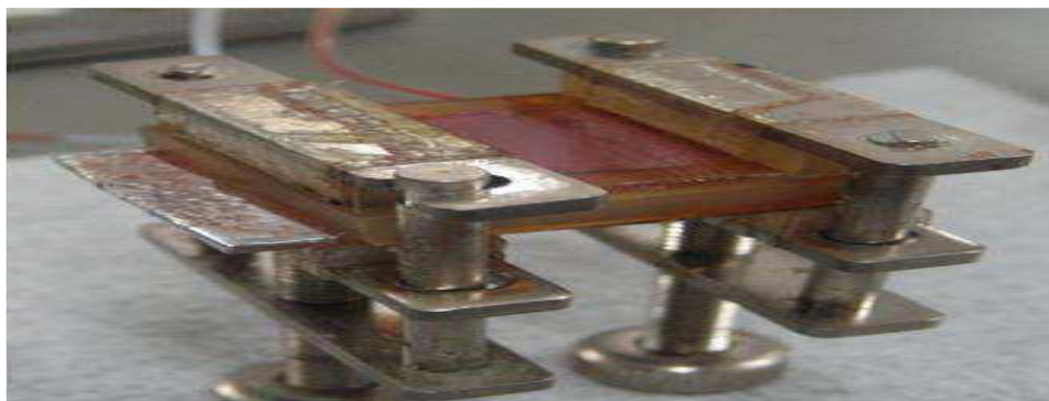
Fig1. Sample structure of photocell
