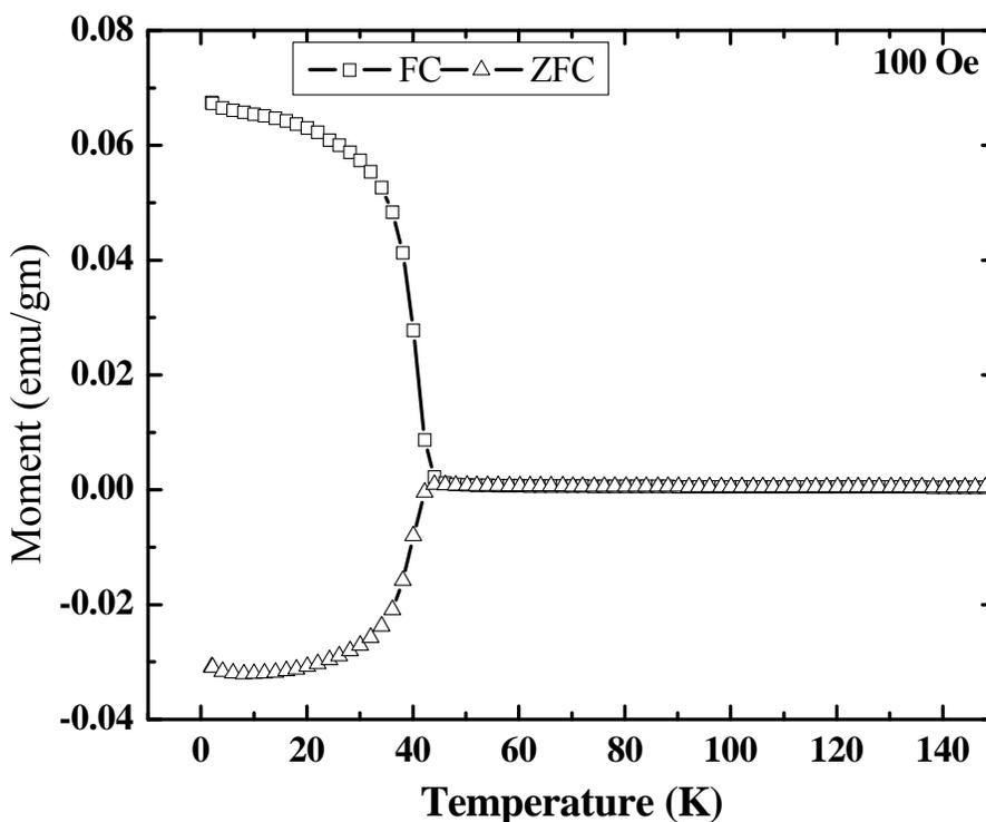
Figure 3. Zero field and field cooled magnetization as a function of temperature for  $(\text{Sr}_{1-x}\text{Ca}_x)\text{MnO}_3$  for  $x=0.8$  have been measured in a magnetic field,  $H=100\ \text{Oe}$
