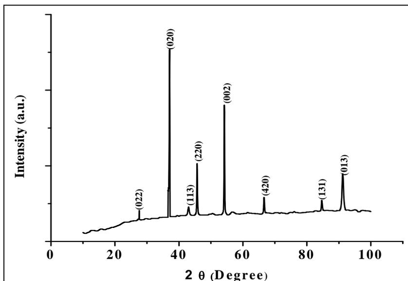
Figure 1. X ray diffraction pattern of  $(\text{Sr}_{0.2}\text{Ca}_{0.8})\text{MnO}_3$  ceramic
