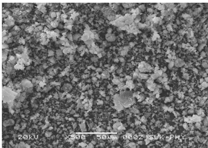
Figure 2. SEM image of  $(\text{Sr}_{0.2}\text{Ca}_{0.8})\text{MnO}_3$  ceramic
