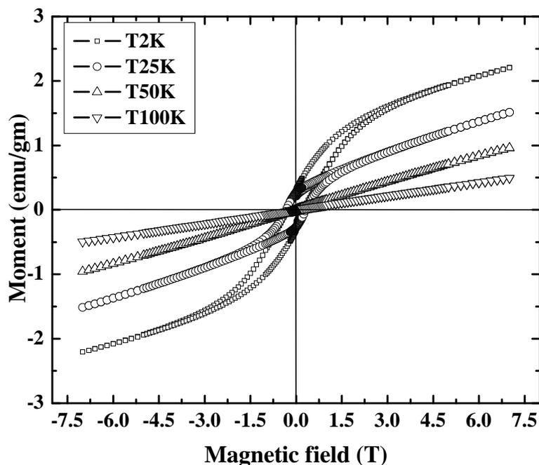
Figure 4. Magnetic-field dependence of magnetization at different temperature for  $x=0.8$ .
