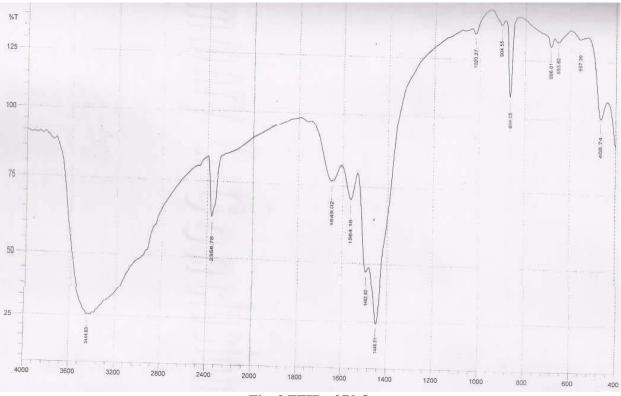
Fig. 3 FTIR of PbO
