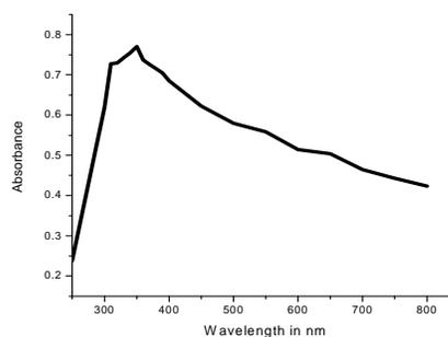
Fig. 2 UV-Vis absorbance spectra for ZnO
