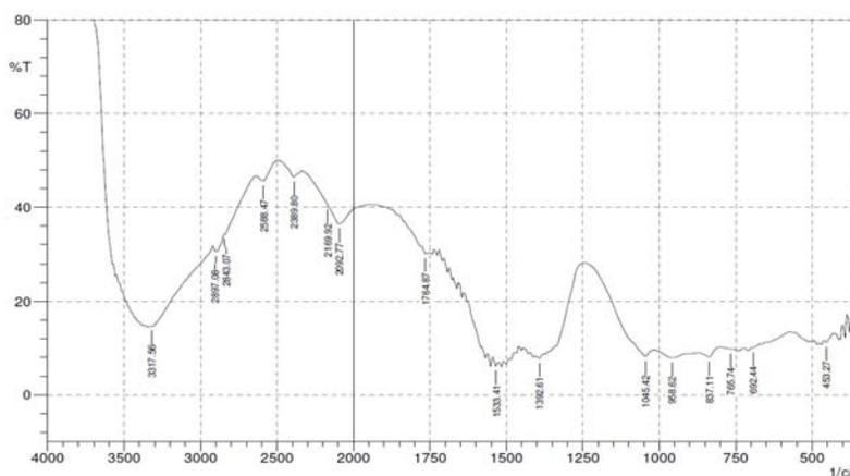
Fig 3. FTIR spectra for ZnO nanoparticle
