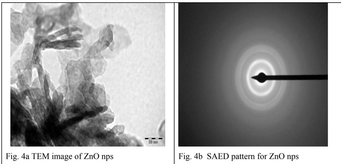
Fig. 4a TEM image of ZnO nps
