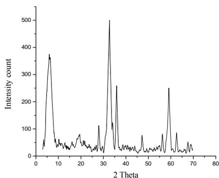
Fig. 1 XRD pattern of ZnO nanoparticle
