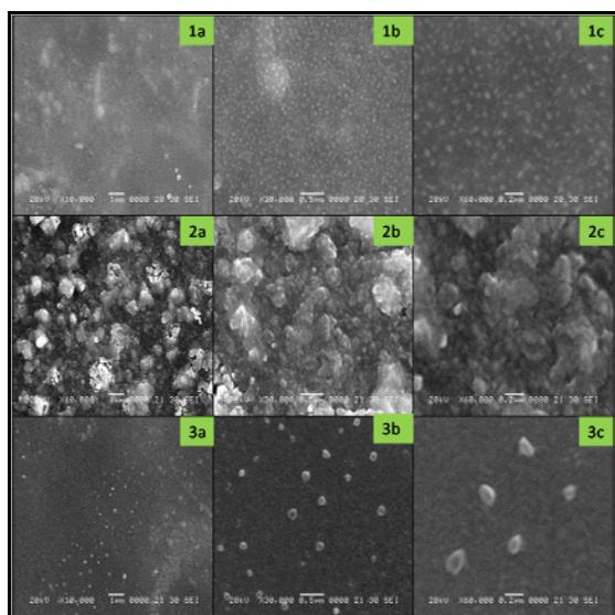
Figure 2. SEM images for 1, 2 and 3 as-prepared CIS films at three different magnifications.
