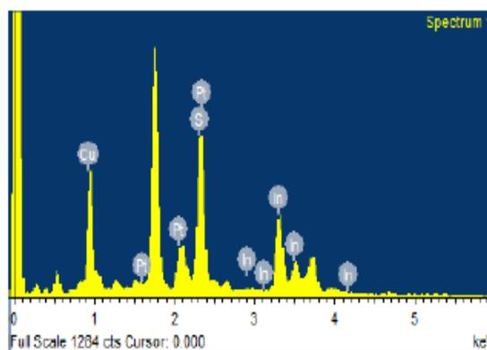
Figure 3 EDAX spectrum for the as-prepared CIS film no. 2
