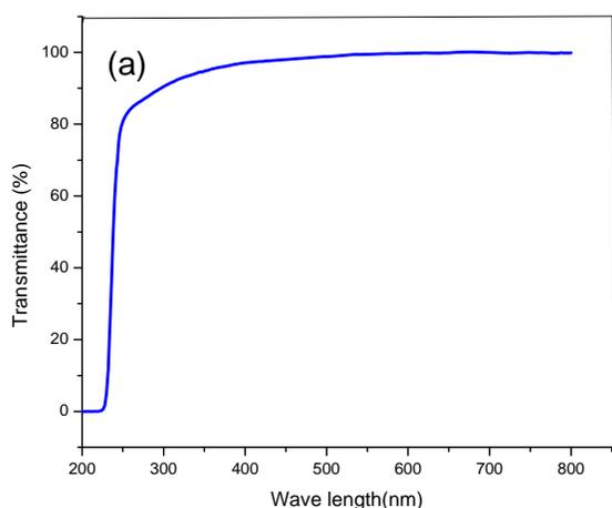
Fig.4 (a). UV- Vis spectrum for transmittance
