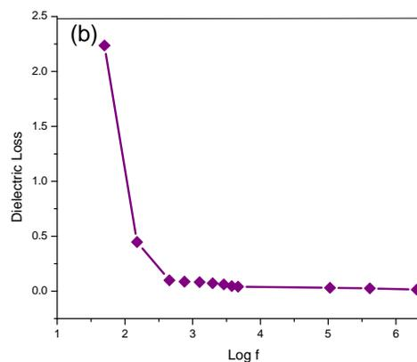
Fig.6. (b) Variation of dielectric loss with frequency
