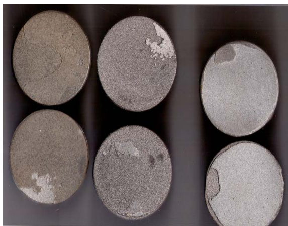
Figure 4 Photograph of tensile bond tested specimens
