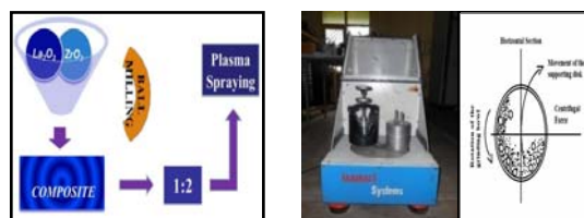
Fig. 1 Experimental set-up in a planetary ball milling
