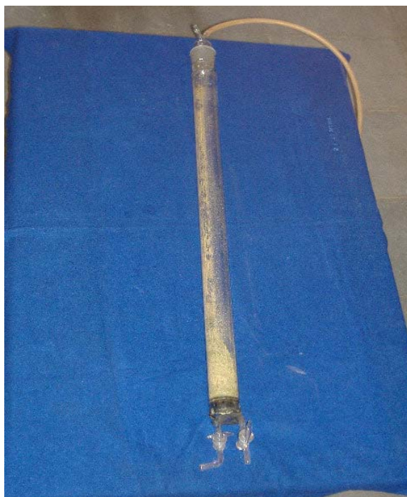
Figure 4 The Packed Bed Reactor Unit
