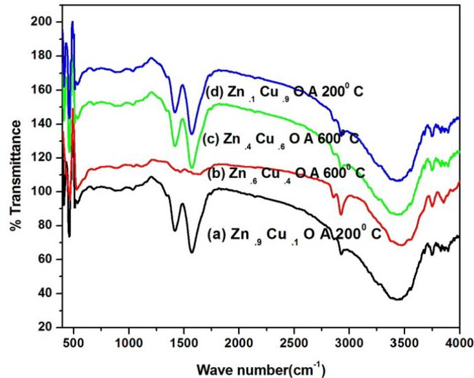
Fig. 3 FT-IR spectrum of Cu doped ZnO nano particles
