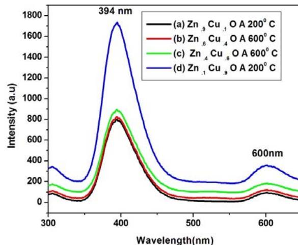
Fig. 5 PL spectrum of Cu doped ZnO nano particles
