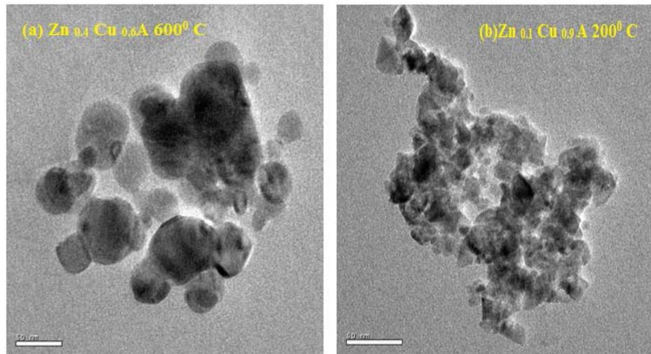
Fig. 2 TEM images of Cu doped ZnO nano particles
