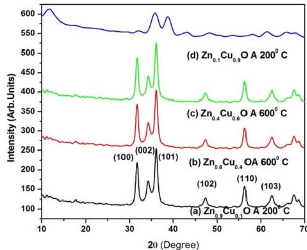
Fig. 1 X-ray diffraction patterns of Cu doped ZnO nano particles
