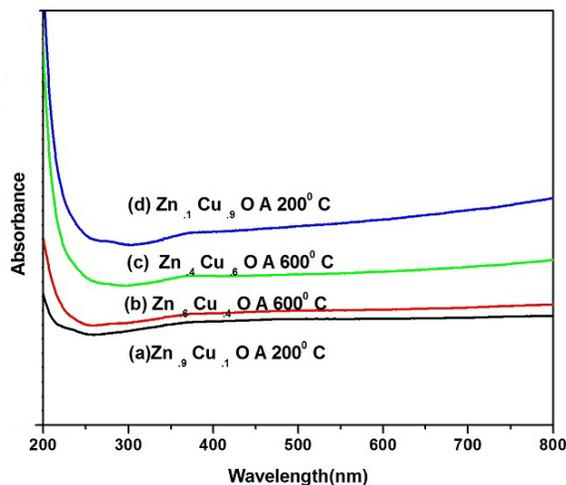
Fig. 4 UV –vis absorption spectrum of Cu doped ZnO nano particles
