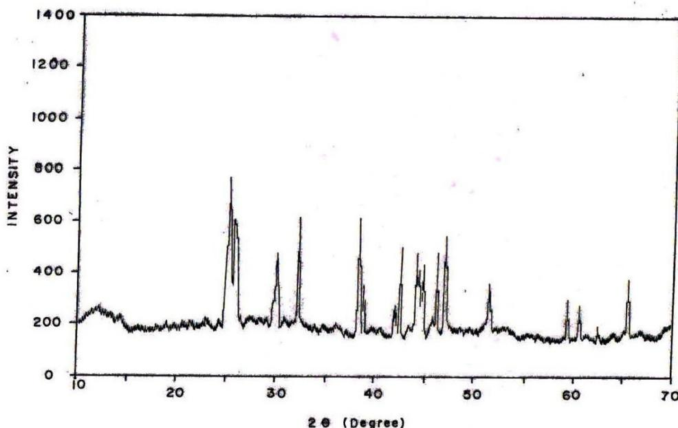
**Figure 1:** X-ray Diffraction pattern of  $\text{La}_2\text{SrBi}_2\text{S}_7$
