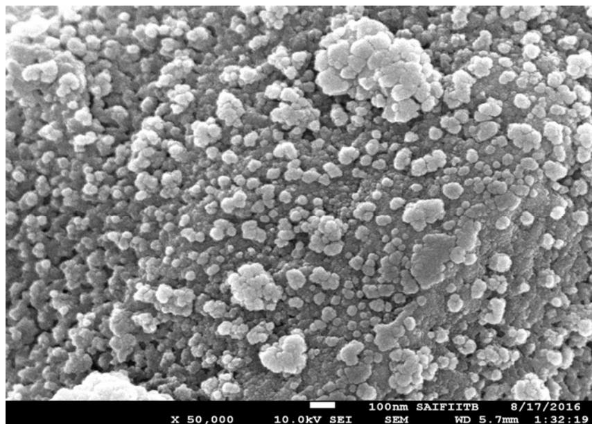
Fig. 3: SEM image of  $\text{Co}_{0.5}\text{Cr}_{0.5}\text{Al}_2\text{O}_4$  thick film.
