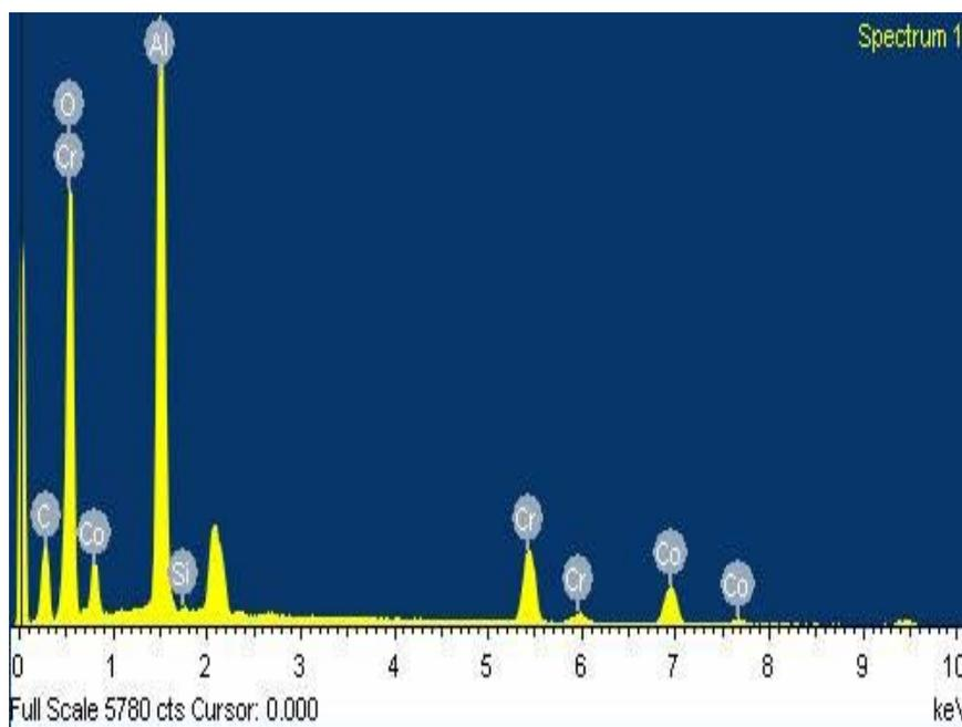
Fig. 4: EDAX spectra of  $\text{Co}_{0.5}\text{Cr}_{0.5}\text{Al}_2\text{O}_4$  thick film.
