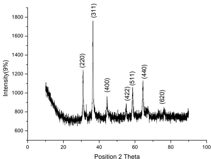
Fig. 1: The XRD pattern of  $\text{Co}_{0.5}\text{Cr}_{0.5}\text{Al}_2\text{O}_4$  sample.
