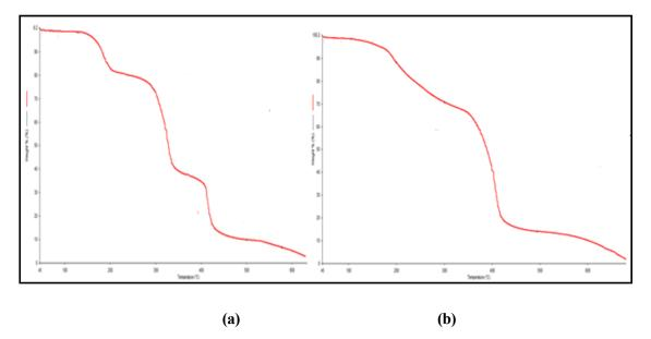
Figure 4: TGA spectrum of Vinyl Ester Resins (a) VER I; and (b) VER II
