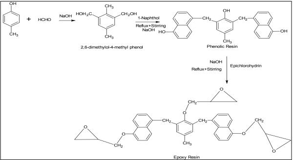
Scheme 1: Reaction pathway for the synthesis of epoxy resin
