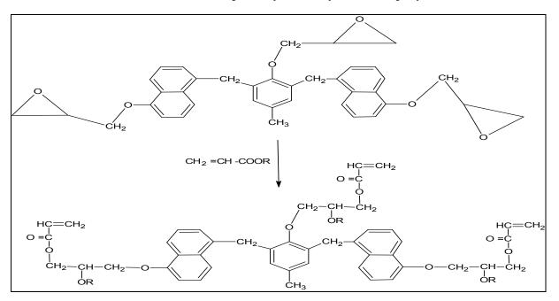
R= -CH<sub>3</sub>, -C<sub>2</sub>H<sub>5</sub> Scheme 2: Reaction pathway for the synthesis of VER resin
