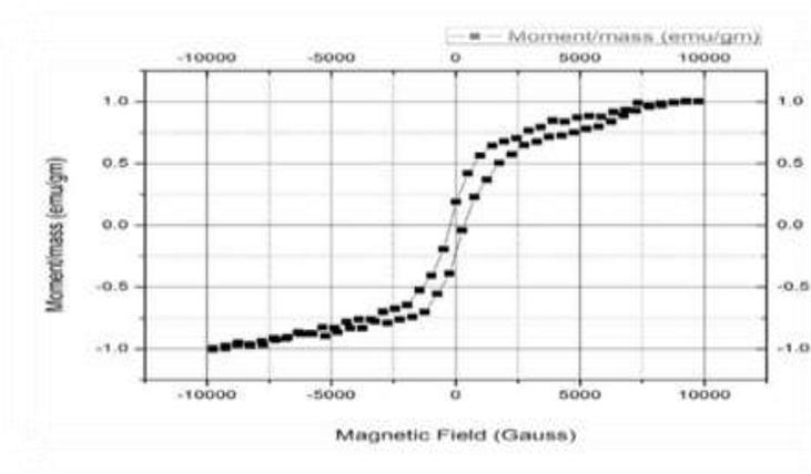
**Fig. 2:** M vs H curve (Hysteresis curve) for the iron oxide (majorly Fe<sub>2</sub>O<sub>3</sub>)
