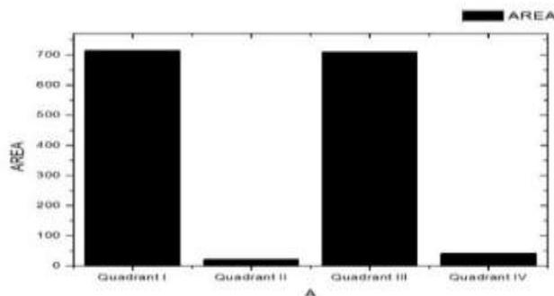
**Fig. 3:** Quadrantwise area distribution of M/H curve
