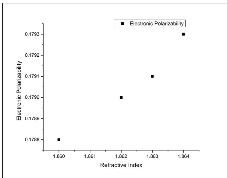
Figure 3. Variation of electronic polarizability with refractive index.
