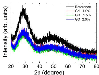
Figure 1 X-ray diffraction pattern of Bi<sub>2</sub>O<sub>3</sub>: Li<sub>2</sub>O: ZnO: B<sub>2</sub>O<sub>3</sub>: Gd<sub>2</sub>O<sub>3</sub> glasses.
