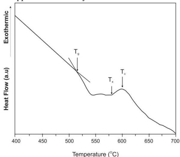
Figure 2. DTA thermogram of powdered ZnLiBiB sample.
