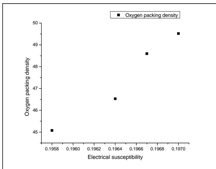
Fig.4. Variation of oxygen packing density with electrical susceptibility.
