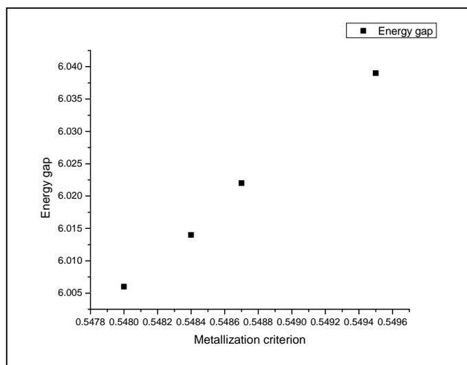
Fig.5. Variation of energy gap with metallization criterion.
