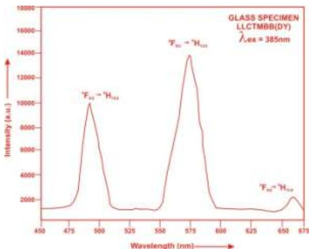
Fig. 4: Fluorescence spectrum of doped with Dy<sup>3+</sup> LLCTMBB glasses.
