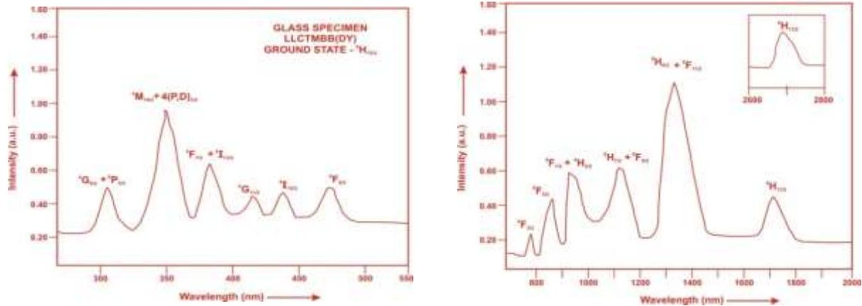
Fig.2: Absorption spectrum of Dy<sup>3+</sup> doped LLCTMBB glasses
